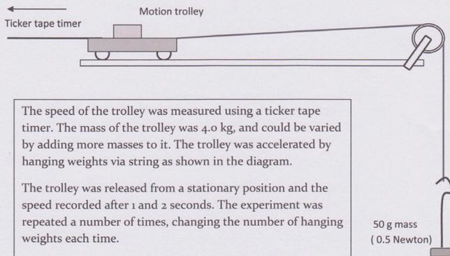
The speed of the trolley was measured using a ticker tape timer. The mass of the trolley was 4.0 kg, and could be varied by adding more masses to it. The trolley was accelerated by hanging weights via string as shown in the diagram.
